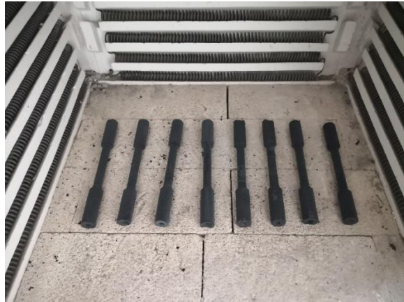
Figure 5: Specimens in Temperature-controlled electric furnace
