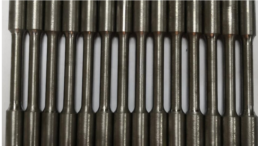
Figure 4: Dumbbell-Shaped Specimens for Tensile Strength Tests
