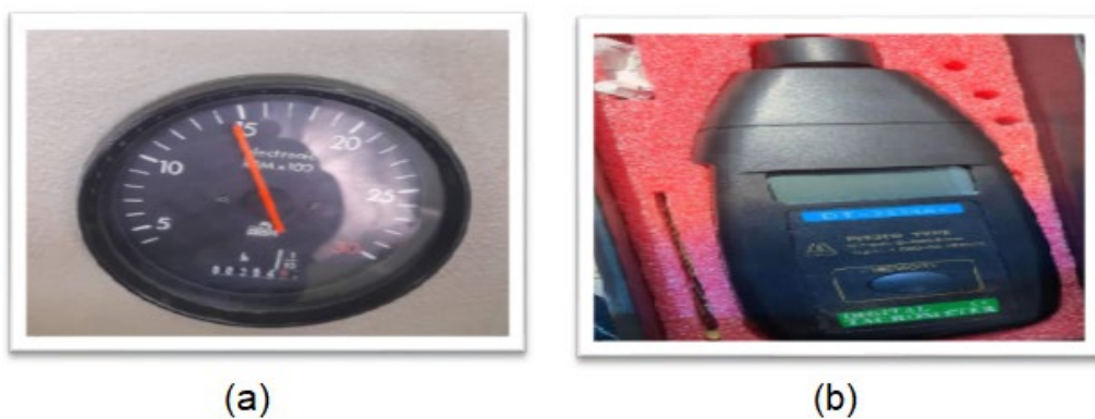
Figure 4.7. Engine speed measurement: (a) engine speed reader, (b) digital tachometer.
