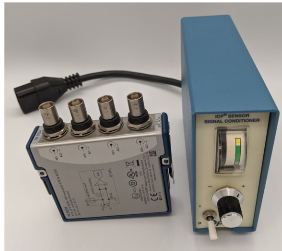
Figure 7.4: Integrated Electronics Piezo-Electric (IEPE) data acquisition systems in various form factors.
