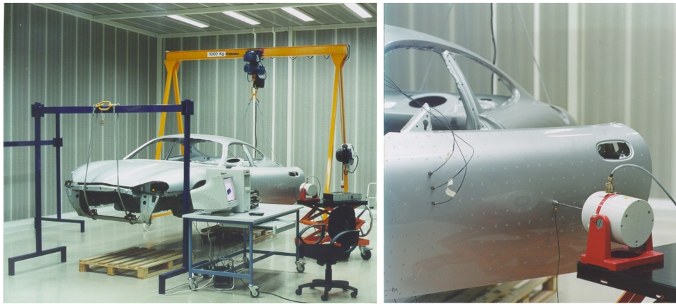
Figure 5.2: Experimental modal analysis of an automotive (Jaguar) body in white, typically done to reduce vehicle noise and vibration harshness a .
