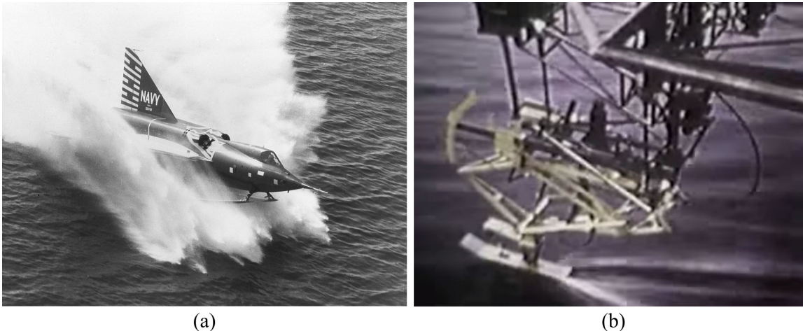
Figure 3.27: The Convair F2Y Sea Dart, showing: a) XF2Y-1 Sea Dart (BuNo 135762) during landing. This airframe disintegrated in mid-air over San Diego Bay, California (USA) during a demonstration flight on November 4th, 1954 killing test pilot Charles E. Richbourg after the airframe limitations were exceeded a , and b) the hydro-skis undergoing extensive testing on a pantograph mounted on a speed boat to study the forces transmitted to the airframe from the hydro-skis b .
