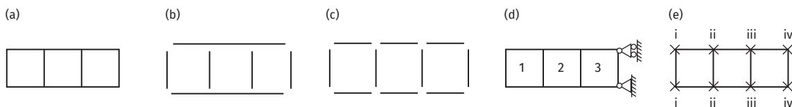
Fig. 8: Numerical modeling approach for the sequential snapping of arrays of units. (a) Schematic of a 1 \times 3 array. (b) An inefficient modeling approach where the base is modeled using two long rods and four short rods, resulting in an imbalance in the number of nodes per rod that would yield inefficient parallel computations. (c) The optimized modeling approach used in this work, with rods of comparable size to ensure a balanced computational load across CPU cores. (d) A target sequential snapping order for the units in the array, with its final boundary condition. (e) The process to achieve sequential snapping: step 1, all base joints marked by crosses are pinned; step 2, all units are snapped simultaneously while the base joints remain pinned; step 3, pins are released in a i, ii, iii sequence, corresponding to the desired snapping order, allowing the global shape to change as the supports are released. To comply with the desired, final boundary conditions in (d), the pins marked by iv become the final boundary conditions.
