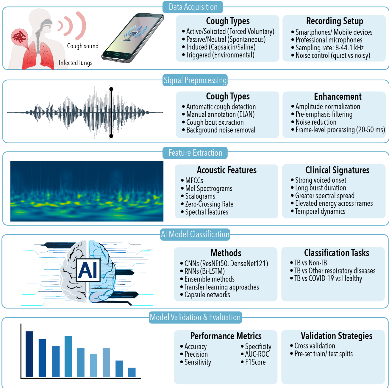
Figure 1. Five-stage cough-based TB diagnostic pipeline encompassing data acquisition, preprocessing, feature extraction, AI classification, and validation.
