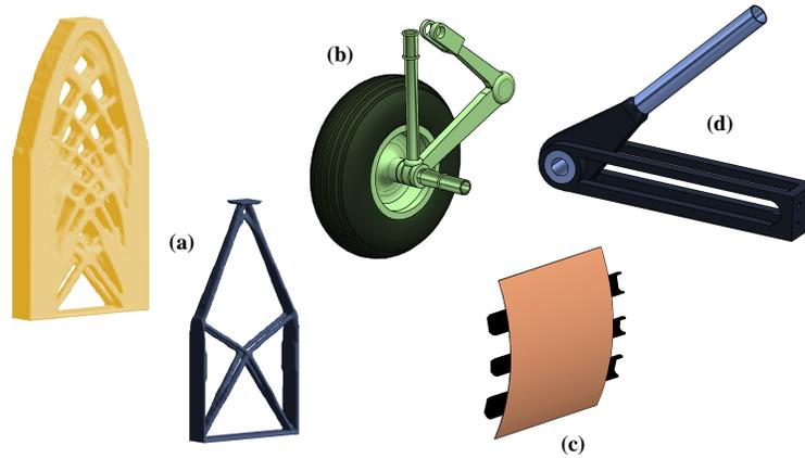
Figure 1: Examples of useful thin walled cylindrical and semi-cylindrical structures including (a) topologically-optimized trusses, (b) aircraft landing gear components, (c) machine structural components, and (d) aircraft skin panels
