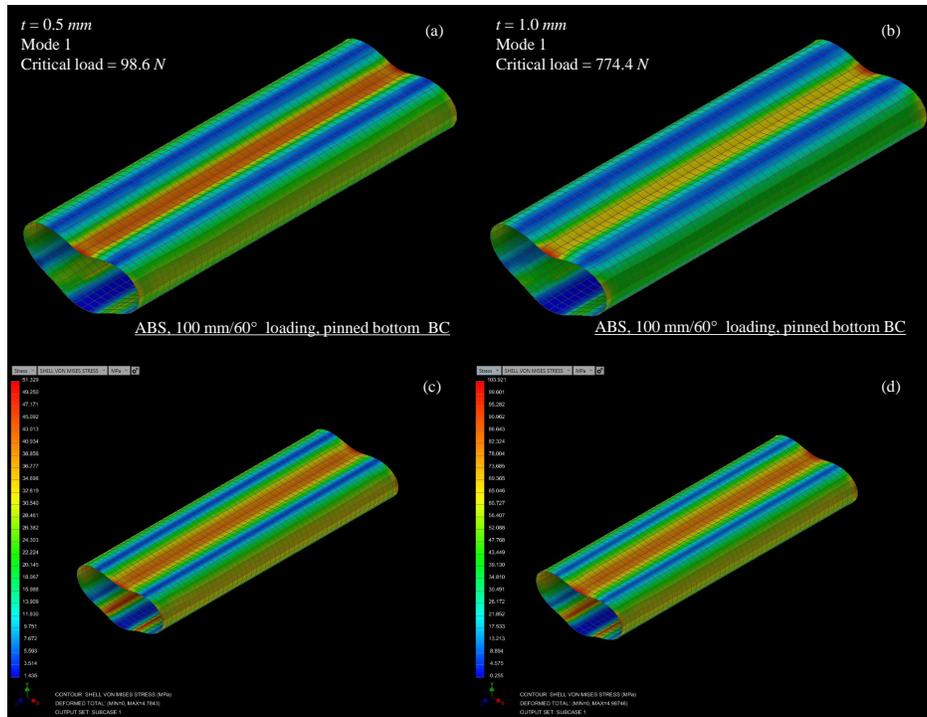
Figure 6: Buckling modes for the (a) thinner and (b) thicker-walled cylinders under the R1 radial loading case, with simple linear static analysis completed at the buckling load of the (c) thin and (d) thick cases to determine if the failure was due to elastic buckling or yielding and then plastic buckling
