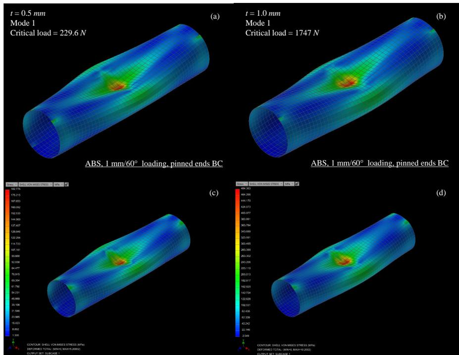
Figure 7: Buckling modes for the (a) thinner and (b) thicker-walled cylinders under the R2 radial loading case, with simple linear static analysis completed at the buckling load of the (c) thin and (d) thick cases to determine if the failure was due to elastic buckling or yielding and then plastic buckling
