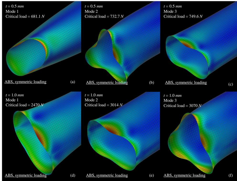
Figure 4: FEA models for symmetric axial loading cases. Shown are 0.5 mm wall (a) mode 1, (b) mode 2, (c) mode 3 and 1.0 mm wall (d) mode 1, (e) mode 2, and (f) mode 3
