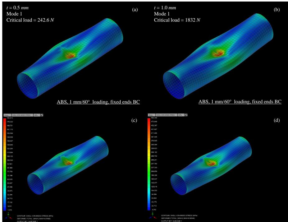
Figure 8: Buckling modes for the (a) thinner and (b) thicker-walled cylinders under the R3 radial loading case, with simple linear static analysis completed at the buckling load of the (c) thin and (d) thick cases to determine if the failure was due to elastic buckling or yielding and then plastic buckling
