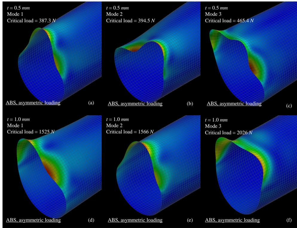
Figure 5: FEA models for symmetric axial loading cases. Shown are 0.5 mm wall (a) mode 1, (b) mode 2, (c) mode 3 and 1.0 mm wall (d) mode 1, (e) mode 2, and (f) mode 3
