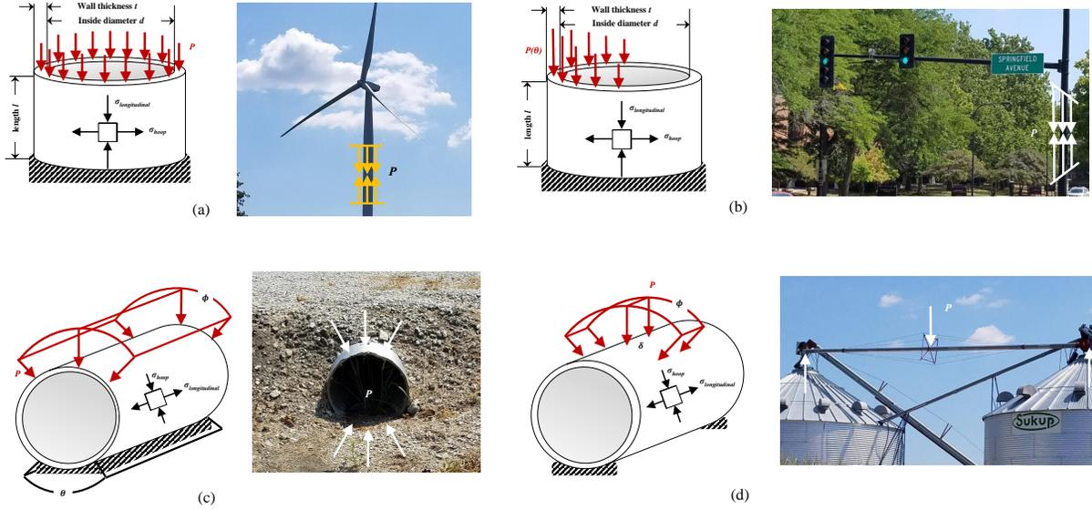
Figure 2: (a) uniform axial load (e.g., wind turbine tower), (b) non-uniform axial load (e.g., traffic light and sign pole), (c) angle-specific uniform radial loading (e.g., drainage culvert), and (d) angle-specific local radial loading (e.g., feed transfer system).
