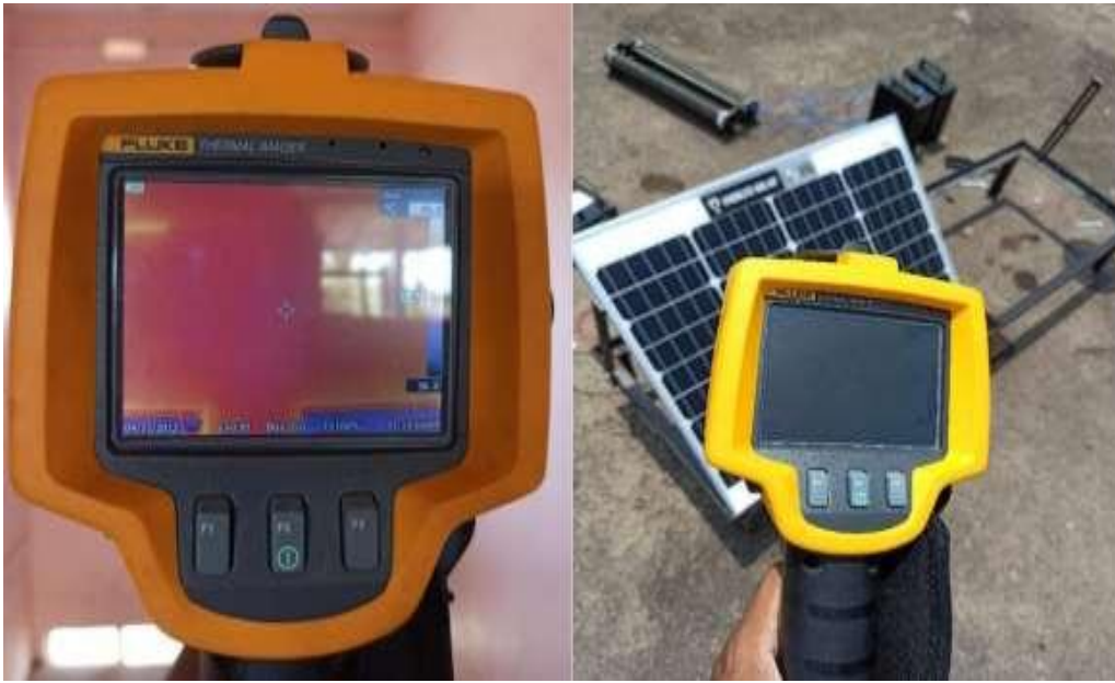
Figure 2: Thermal camera used for measuring the temperature developed on the PV panel
