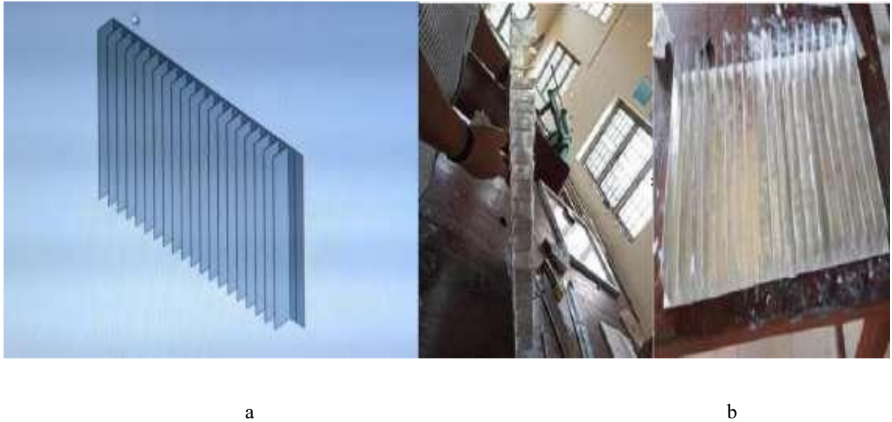
Figure 4 (a) designed fins (b) Fabricated fins made up of aluminum
