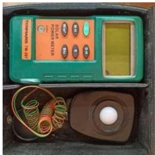
Figure 5: A pyranometer was used to measure the solar irradiance
