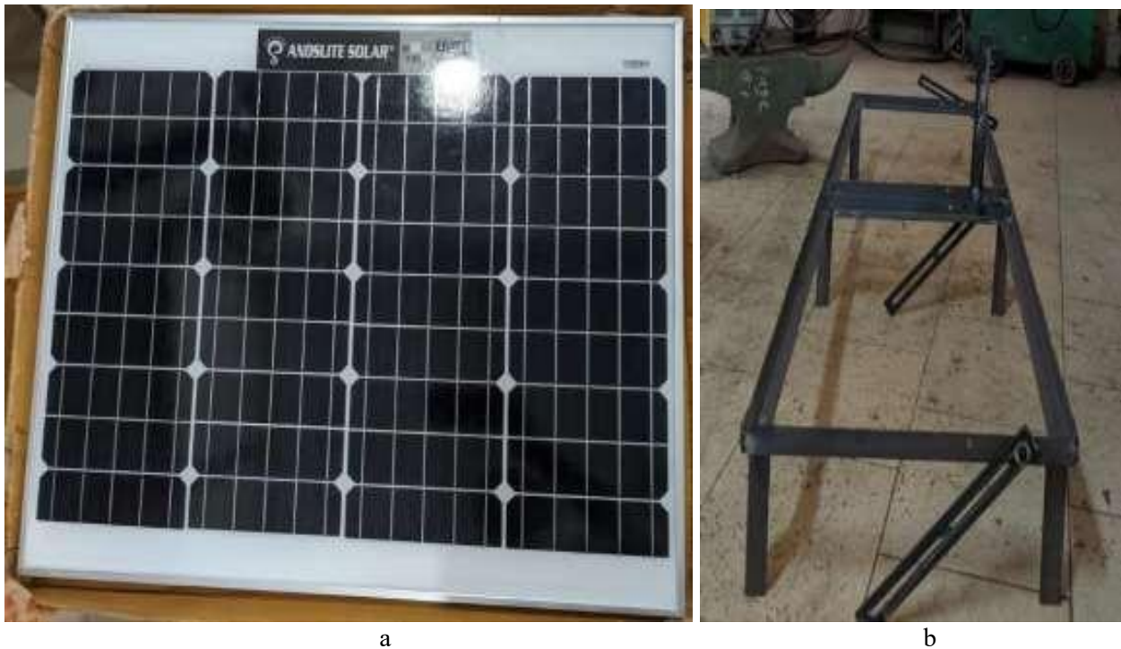
Figure 1. (a) 50 W, 12 V photovoltaic panel; (b) tiltable stand used to position the photovoltaic panel.
