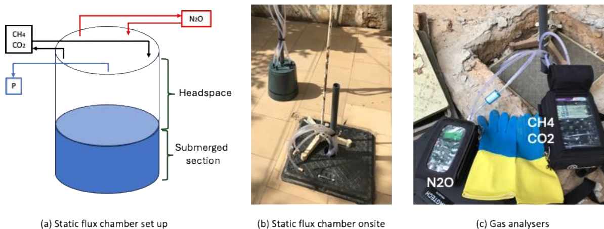
Figure 4. Static flux chamber used for assessing GHG emissions from onsite sanitation containment units. (a) Static chamber diagram with ports for gas sample collection and pressure measurements; (b) Static flux chamber used on site and its deployment in a “holding tank” through an inspection manhole in Senegal; (c) Portable field gas analysers.
