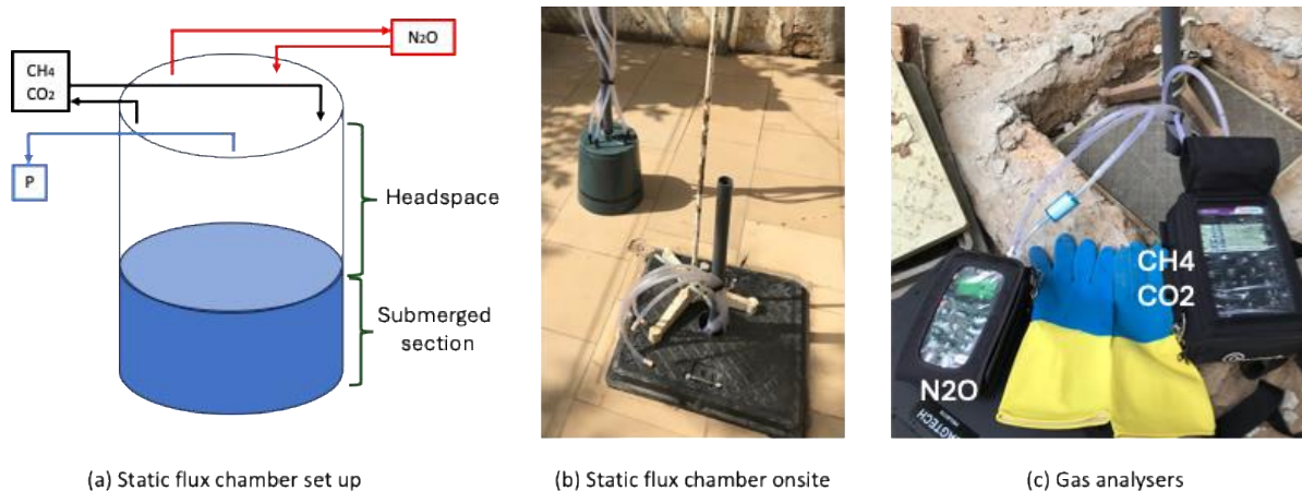
Figure 8. Static flux chamber used for assessing GHG emissions from onsite sanitation containment units. (a) Static chamber diagramme with ports for gas sample collection and pressure measurements; (b) Static flux chamber used on site and its deployment in a “holding tank” through an inspection manhole in Senegal; (c) Portable field gas analysers.
