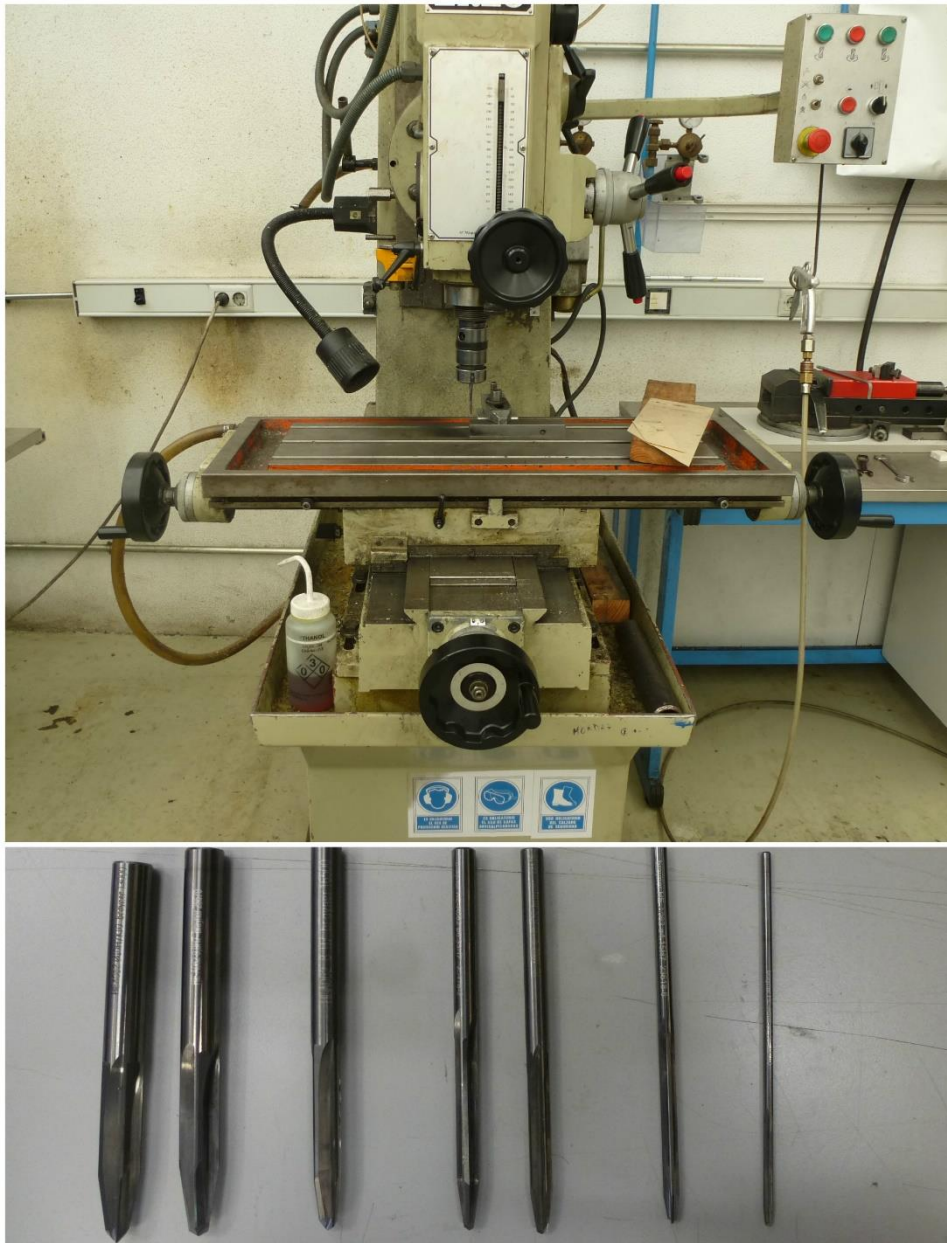
Figure A-11. Drilling machine and reamers used during the drilling stage.
