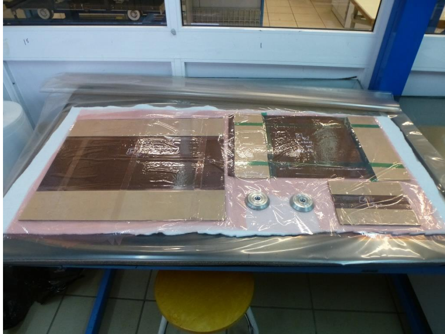
Figure A-8. Second vacuum bag for the curing of the tabbing adhesive.
