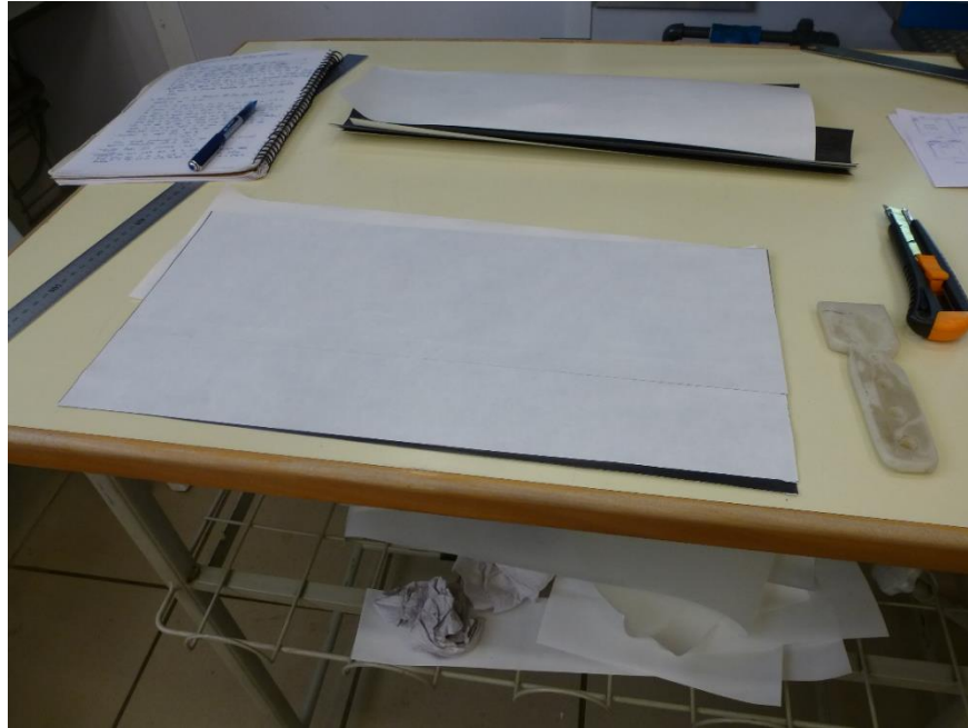
Figure A-2. Panel's laminae lay-up process.
