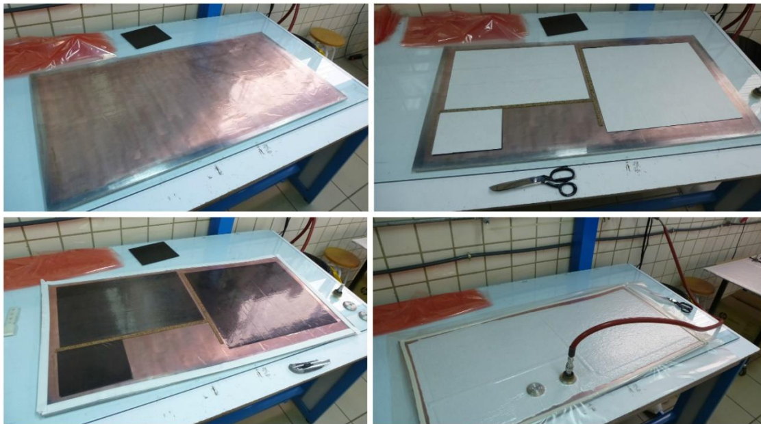
Figure A-3. Vacuum bag fabrication procedure. a) top left, b) top right, c) bottom left, d) bottom right.
