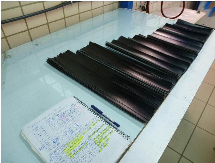
Figure A-1. All the laminae cut from the unidirectional tape ready to be piled.
