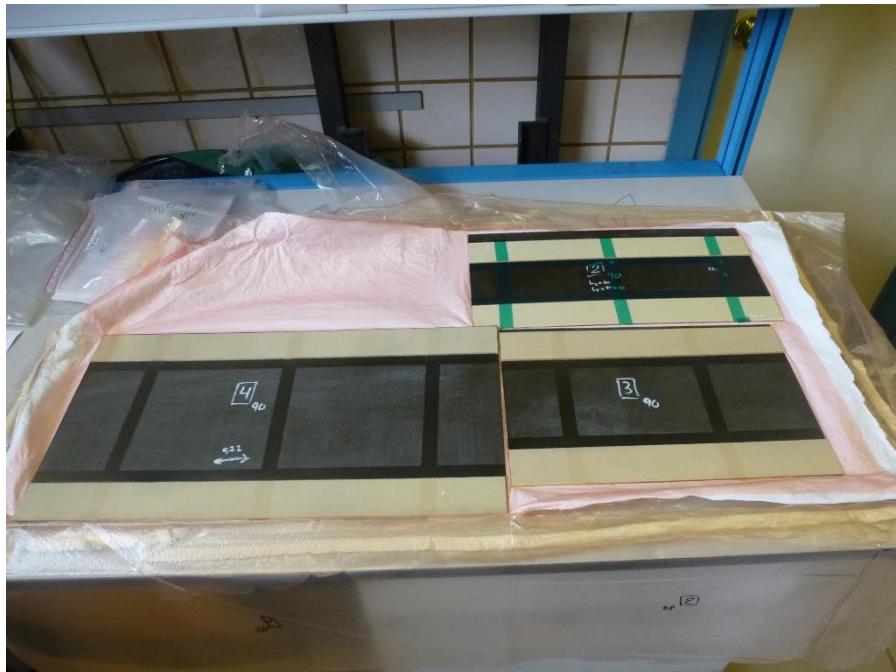
Figure A-9. Panels after the curing of the adhesive in the autoclave.
