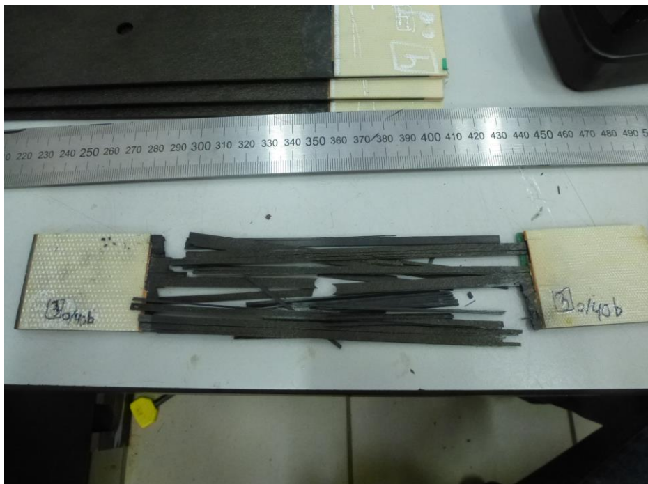
Figure A-14. Explosive failure of P3-0°-40-b.
