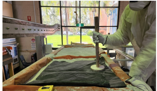
Figure 2. Placement of MAB-1 simulant prior to compaction.
