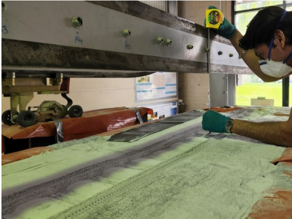
Figure 4. Surface settlement monitoring using physical measurements.
