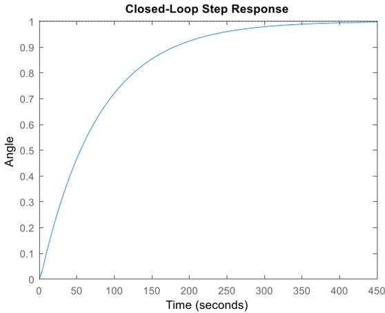
Fig.6. Negative feedback closed loop system step response
