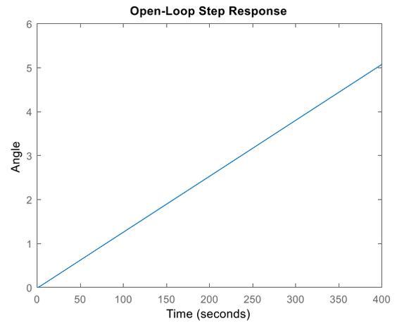
Fig.4. Open loop step respnse
