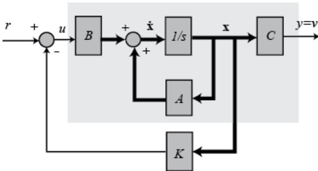
Fig.9. Closed-loop system with full state feedback controller
