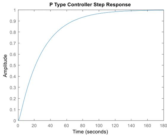
Fig.7. Closed loop system with P controller step response
