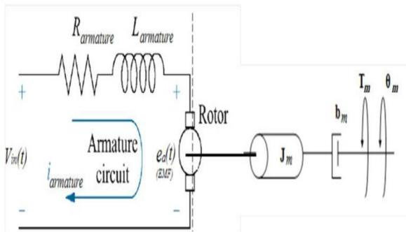
Fig.1. Equivalent representation of PMDC motor electromechanical component
