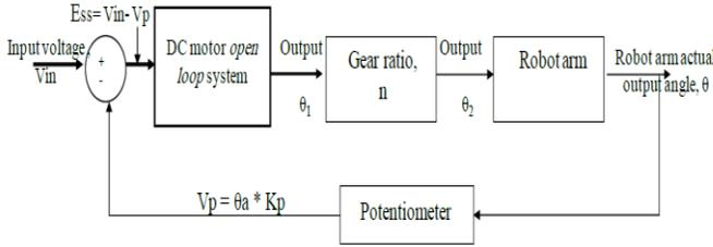
Fig.5. Negative feedback closed loop system block diagram
