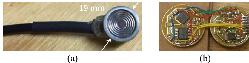
170 Figure 3. Earth pressure cell: (a) Plan view; (b) Internal 3-axis accelerometers. 171
