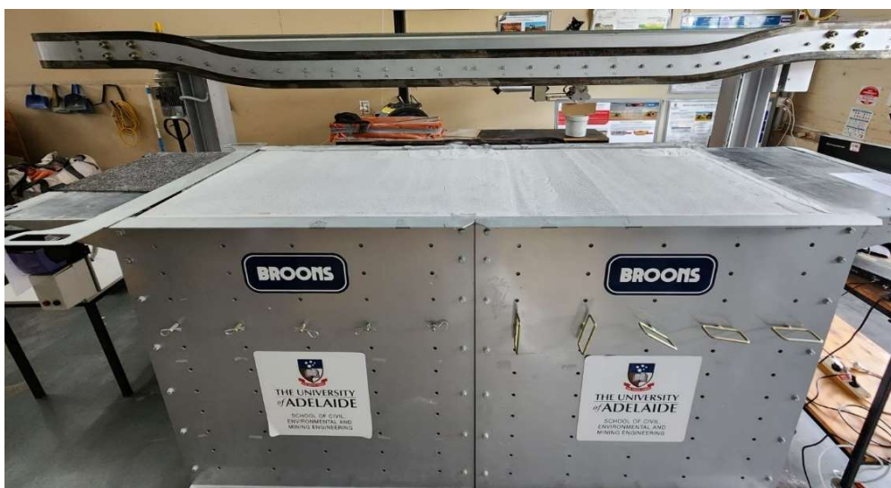
Figure 1. Test facility setup after lunar highland regolith simulant placement.
