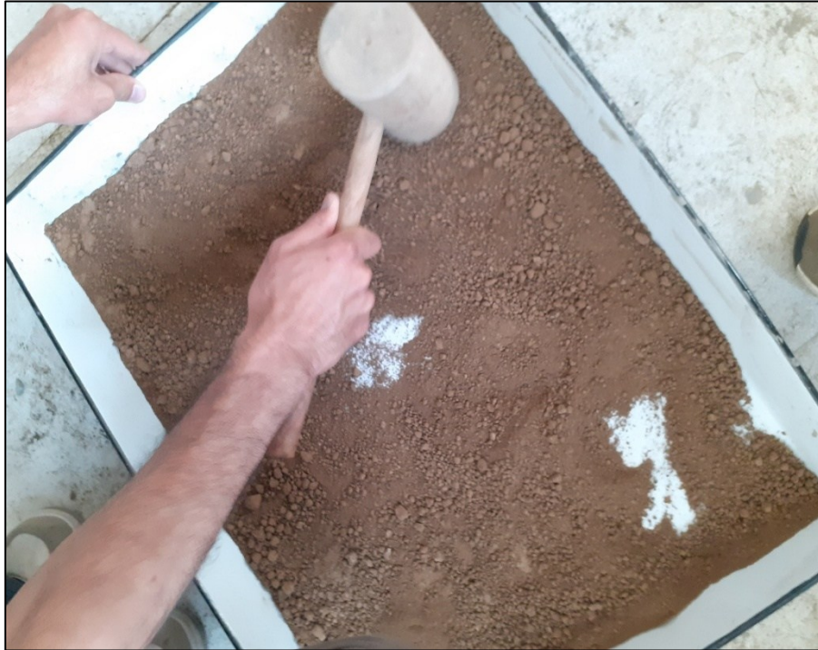
Fig. 2 Pulverization of soil using wooden hammer to ensure a uniform texture
