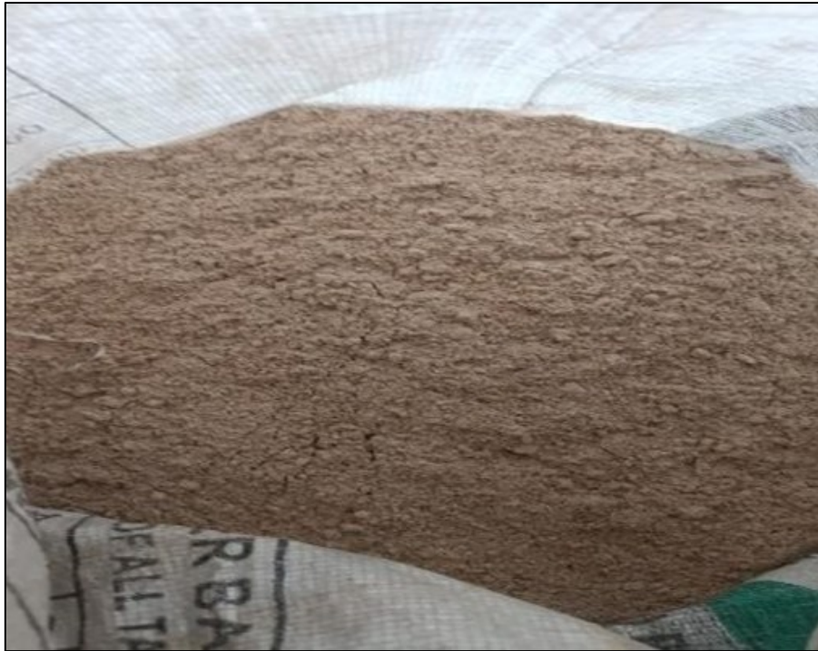
Fig. 5 Kashmir rice husk selected for soil stabilization
