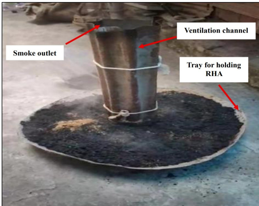
Fig. 6 Burning of rice husk to activate its pozzolanic properties
