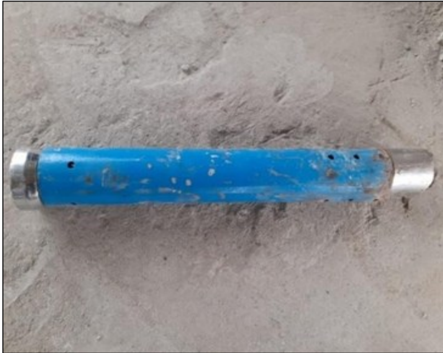
Fig. 8 Proctor hammer of 2.5 kg used for manual compaction of the mixture in the mould
