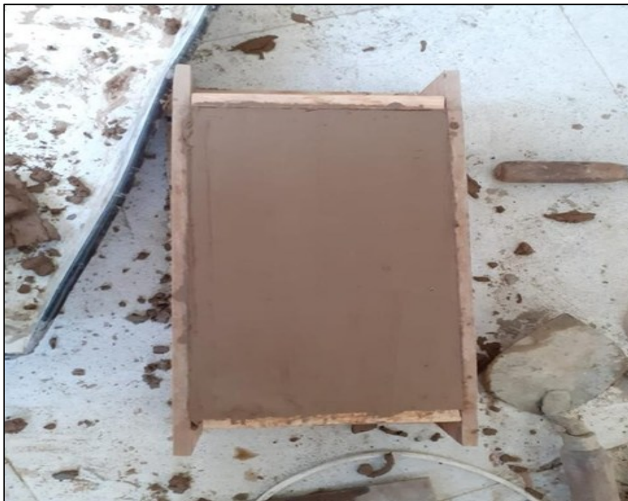
Fig. 9 Prepared sample of compressed stabilized earth block in mould of dimensions 300 mm x 150 mm x 100 mm
