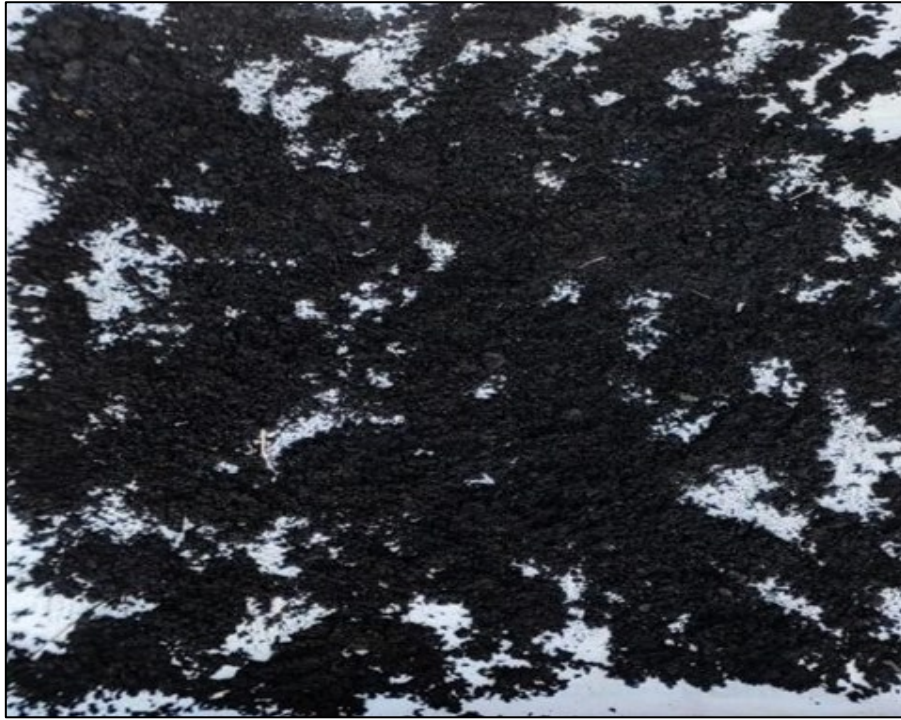
Fig. 7 Rice husk ash obtained after burning of rice husk
