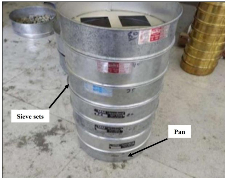
Fig. 1 Sieve sets used to perform sieve analysis of the aggregates
