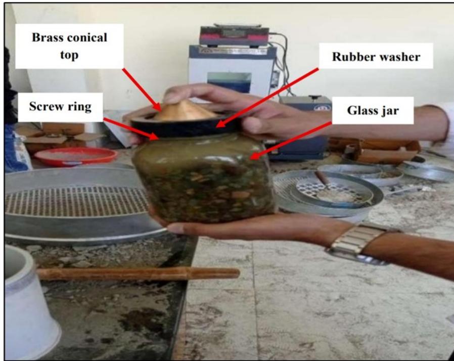
Fig. 2 Pycnometer apparatus used to determine specific gravity of the aggregates
