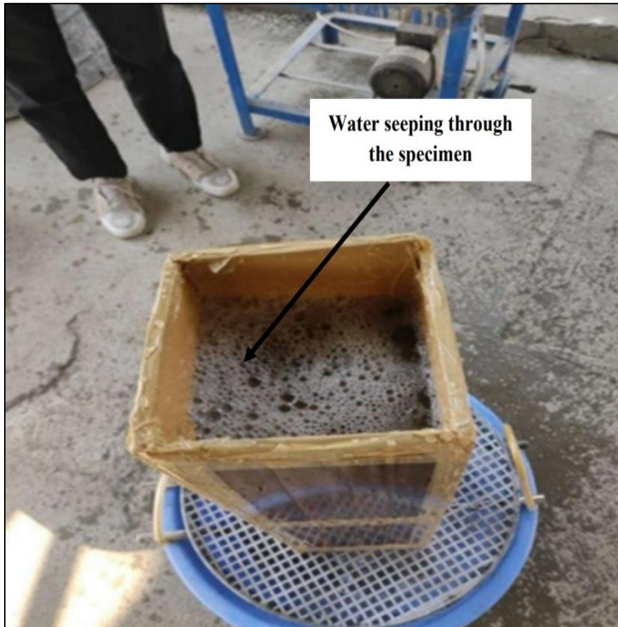
Fig. 7 Passing of water through the pervious concrete specimen
