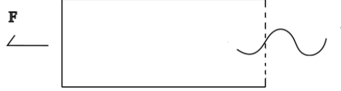
Fig. 5 Schematic of the "Virtual Wire" model. The solid lines represent the physical open-circuit coil. The red dashed line represents the "Virtual Wire" used for theoretical analysis. Together, they form a virtual closed loop for calculation and analysis
