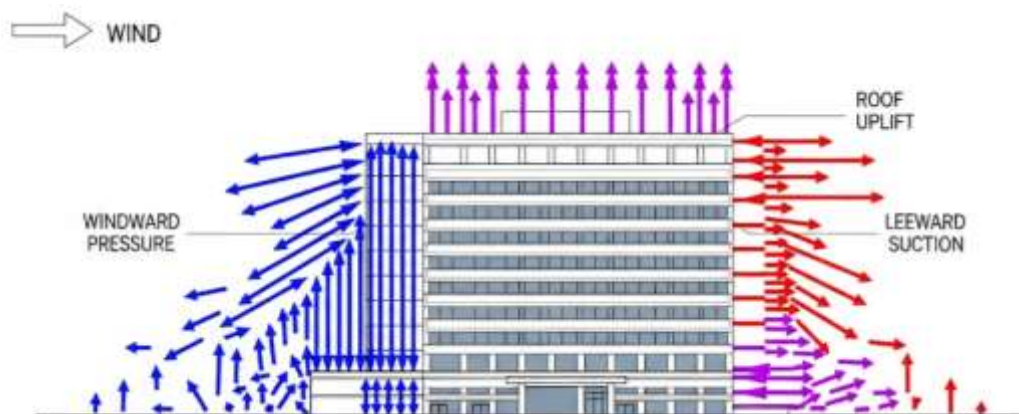
Figure 17 Wind Pressure Distribution Pattern on Walls and Flat Roofs
