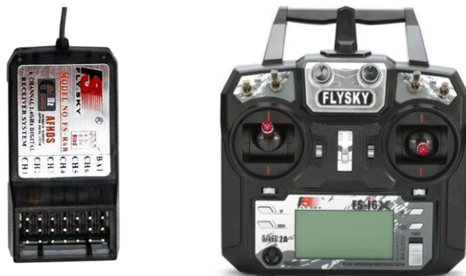
Figure 11. Remote controlling system
