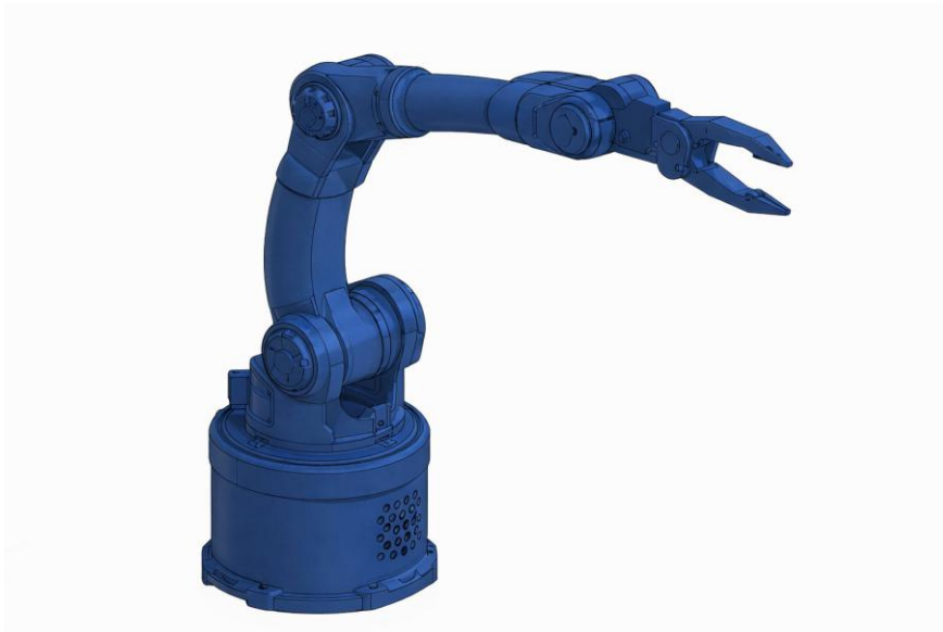
Figure 4.2: CAD model of an articulated six-axis robotic arm configured for sheet metal cutting applications
