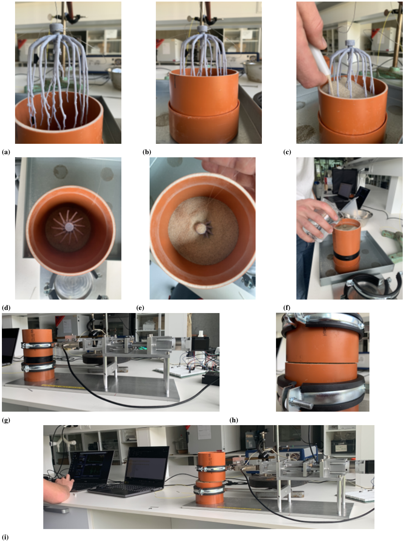
Fig. 4. Main stages in specimen preparation and installation in the RSSA: (a) root system positioned in the lower half of the split PVC pipe; (b) root embedment depth adjusted to the target level; (c) sand poured into the first half of the cylinder; (d) second half of the PVC pipe assembled and secured with tape; (e) sand placement completed to the target height; (f) water added and specimen left at room temperature for 1 h; (g) PVC section placed in the RSSA groove; (h) tape removed and a gap is ensured along the shear plane; (i) direct shear test started with RSSA measurements and fiber-optic readings.
