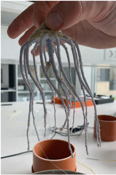
Fig. 5. Post-test configuration of the 3D-printed synthetic root system, showing bending and distortion of the branches after shearing.
