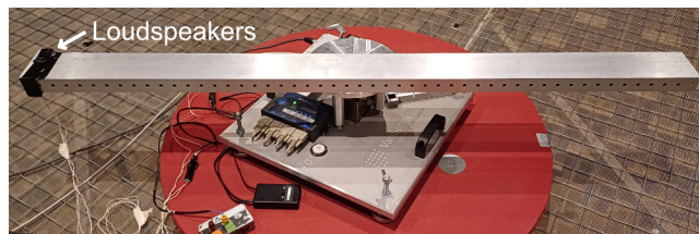
FIG. 9: The prototype antenna with attached loudspeakers, placed on the turntable.
