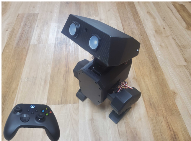
Fig. 4. Hardware setup of the Open Duck Mini V2 platform and controller used in the experiments. The robot is equipped with onboard computation and actuators for real-time locomotion control.
