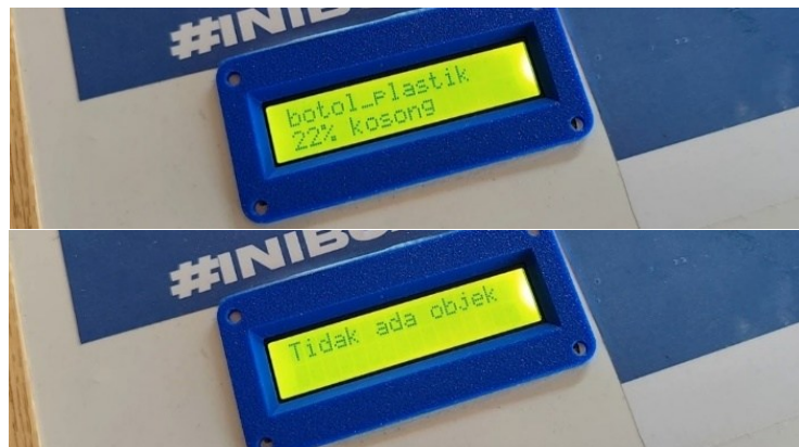
Figure 14. LCD 16x2 I2C Testing
