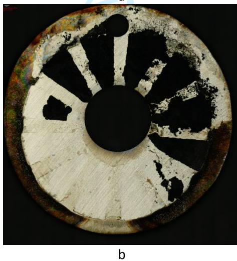
45 46 47 48 49 50 51 52 53 54 55 56 57 58 59 60 FIG. 8 – (a) Current density and temperature as a function of immersion time of UNS S39274 in natural seawater at an applied potential of E_{\text{App}} = +300 \text{ mV}_{\text{SSE}} and (b) visual appearance after 110 days of exposure.
