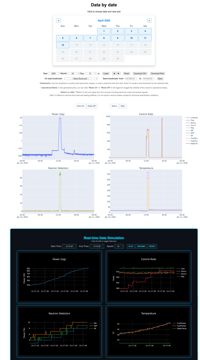
Figure 2. Data by Date interface of the NTW platform. The upper panel provides synchronized time-series visualizations for detailed analysis of reactor operational data, while the lower panel enables dynamic replay of reactor behavior, allowing users to examine transient responses and operator actions in a time-resolved manner.
