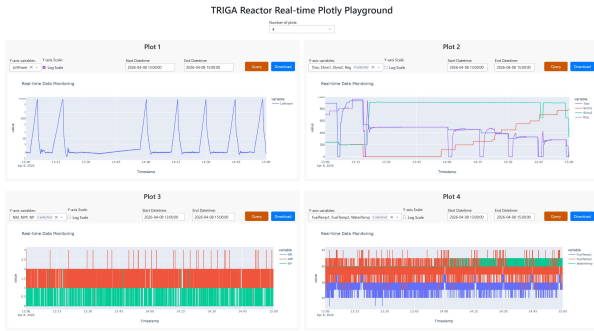
Figure 3. Data Playground interface of the NTW platform, enabling user-defined querying and visualization of reactor operational data. Multiple plots can be generated simultaneously to support flexible analysis of correlations and trends across different reactor parameters.
