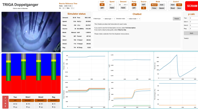
Figure 4. Interactive reactor simulator of the NTW platform. The interface replicates the NETL TRIGA control panel and integrates real-time visualization of reactor state, control rod positions, and system parameters, along with auxiliary components such as a status panel and chatbot interface to support interactive operation and training.
