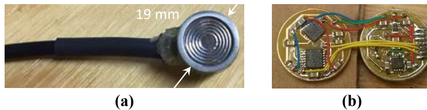
265 Figure 3. Earth pressure cell: (a) Plan view; (b) Internal 3-axis accelerometers.
