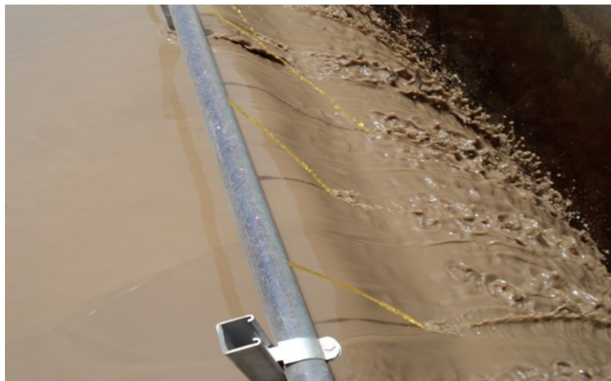
Plate 2: The application of the Coagulant to the raw water
