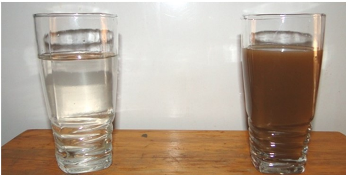
Plate (1): Turbidity in Raw Water
