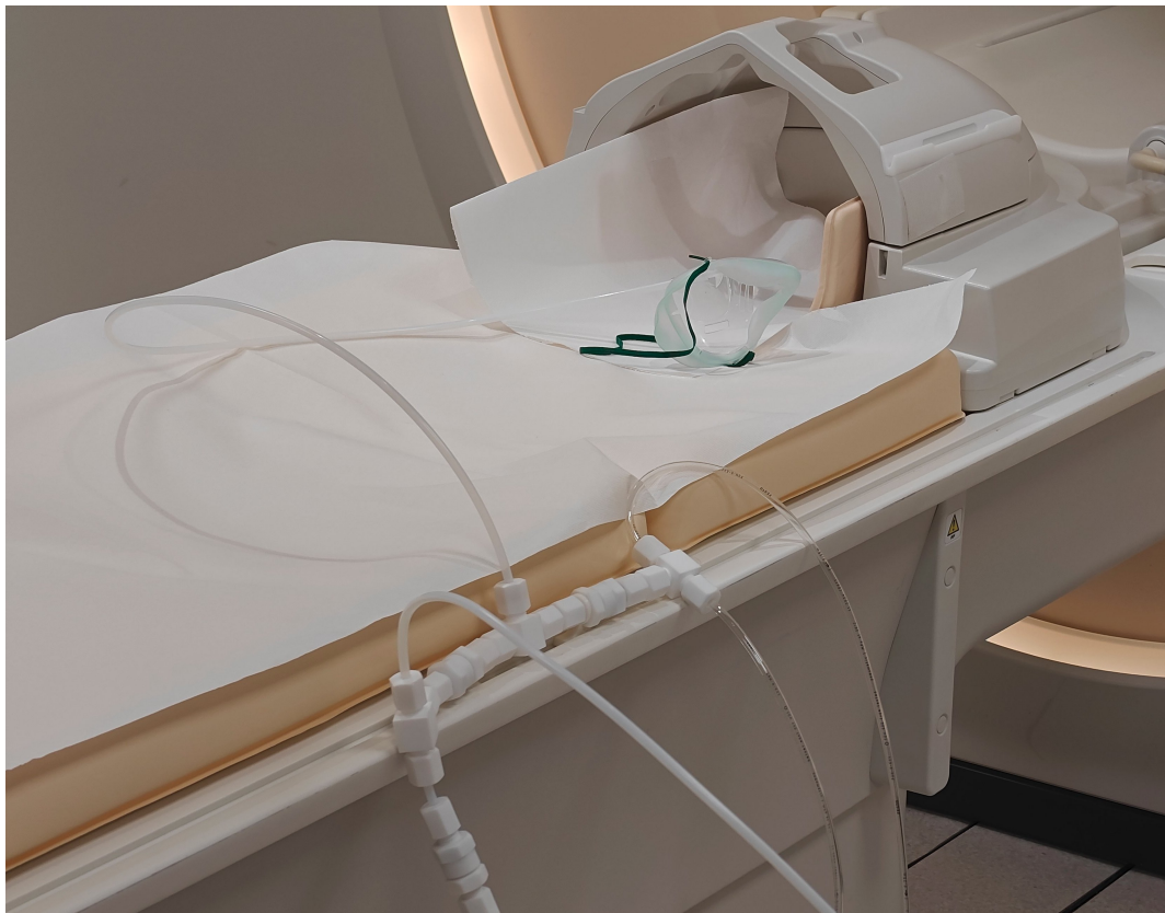
Fig. S5: Position of the vacuum-switch in the MRI room. Shown here is the position at the bore entrance. The picture does not show the table inside the MRI bore, which is the case for the test.
