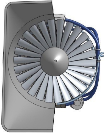
Fig. 15. Front view of the engine showing the turbine blades.
