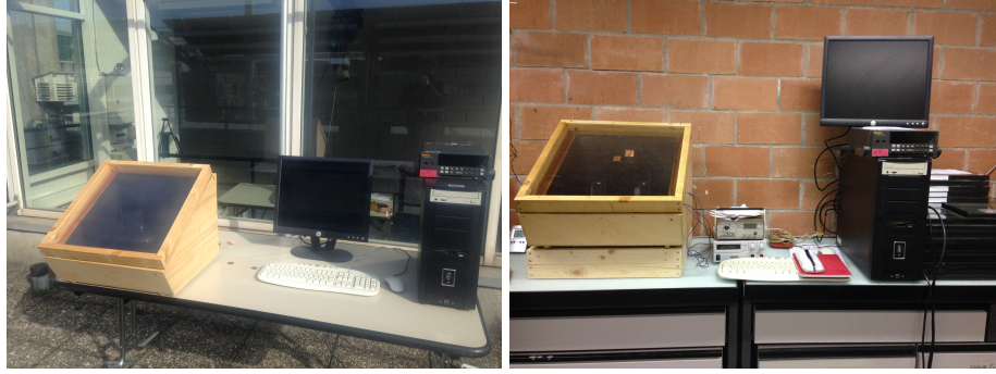
Figure 4: Experimental setup for temperature measurements under solar irradiation (left) and for determination of the U -value (right)
