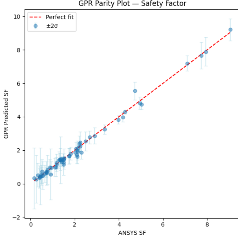
Figure 1: GPR parity plot — predicted vs ANSYS SF with \pm 2\sigma uncertainty bounds
