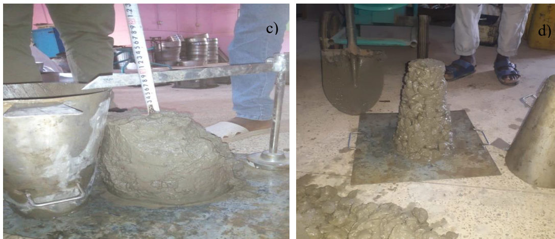
Fig. 2 a grading of fine aggregate (sand), b grading of coarse aggregate (CC and OS), c slump measurement of CC, d slump measurement of OS
