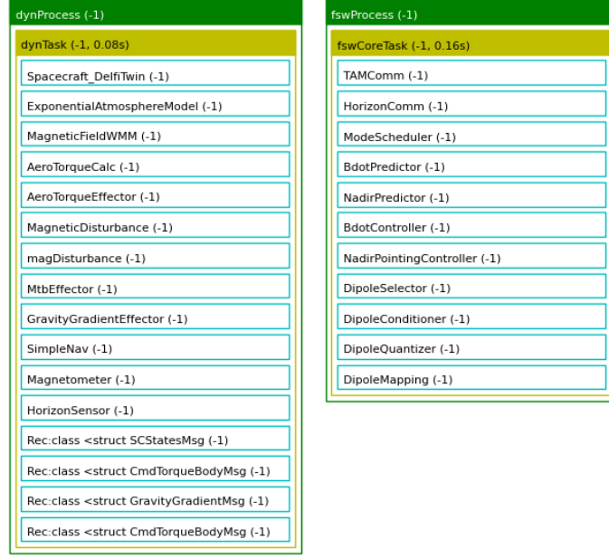
Figure 5.5: Integrated closed-loop Basilisk simulation architecture for nadir pointing mode
