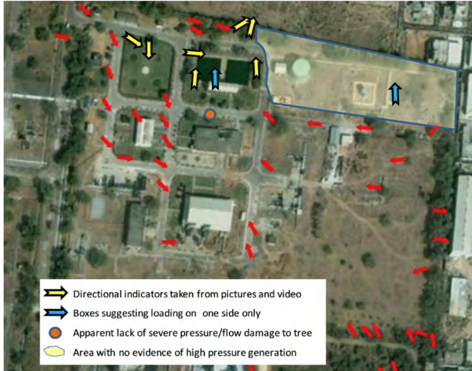
Figure-S 2.1 Jaipur directional indicators in the Pipeline Division area and area without apparent pressure generation. Figure taken from [4]. The partial transparency through the yellow area shows the green tank, and the wall that is not damaged is the northern edge of the blue area. The main firewater pump house is just south of the firewater ponds.
