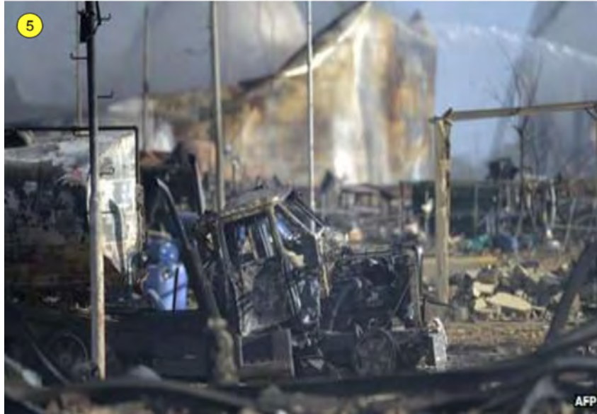
Figure-S 4.9 Damage to truck inside the lube oil plant. Damage suggests detonation.
