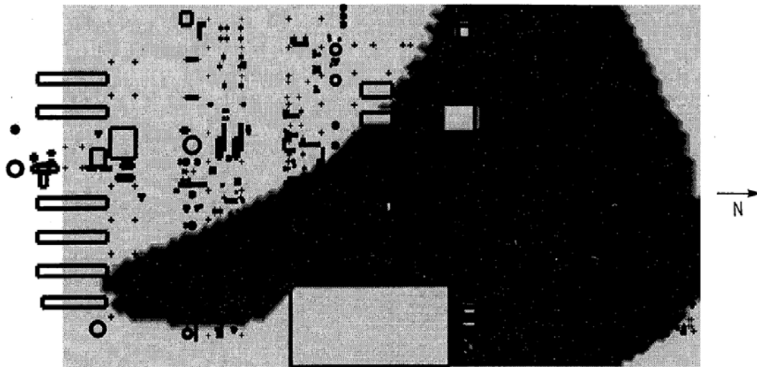
Figure-S 13.3 Naphtha cracker unit with cloud contour. (Reproduced with permission of [29].)
