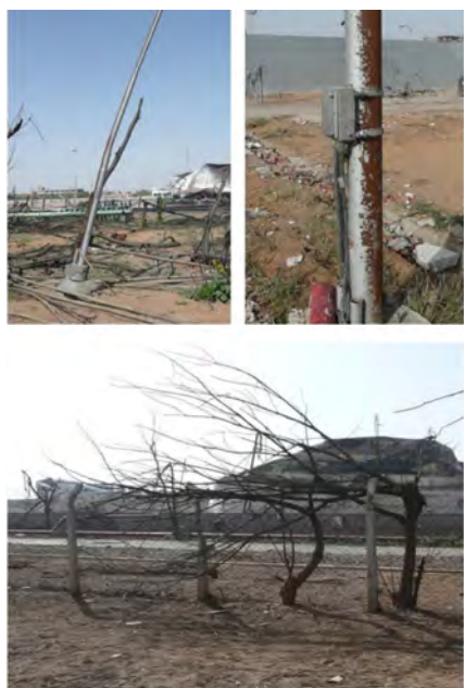
Figure-S 2.3 Examples of directional indicators: bent trees and scoured poles [4].
