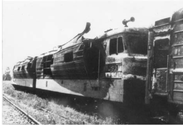
Figure-S 7.7 Internal explosion(s) evidenced by the barrel like shape of coaches and locomotives [15].
