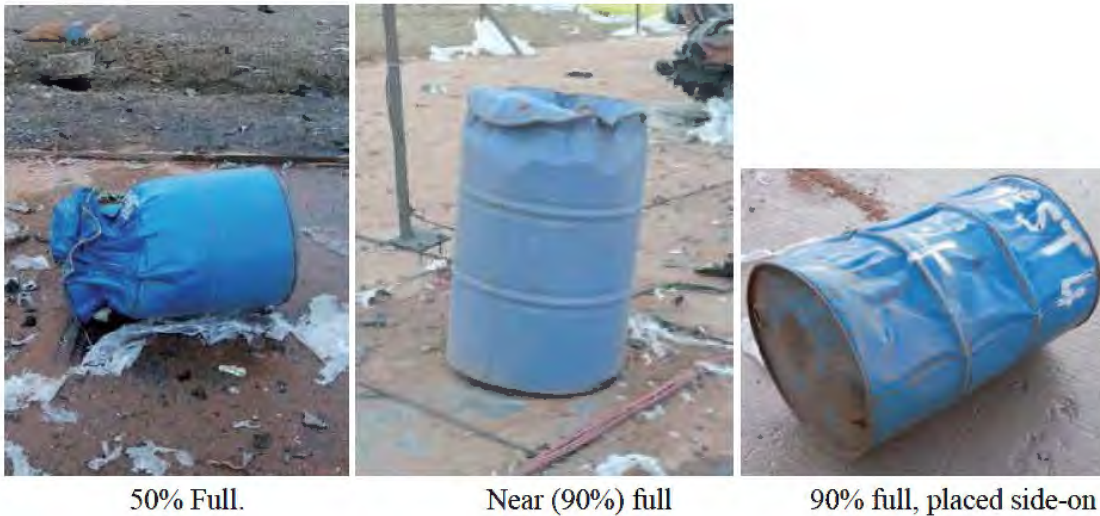
Figure 4.3 Damage to standard steel oil drums placed inside the detonation, (photographs reproduced from [32]).
