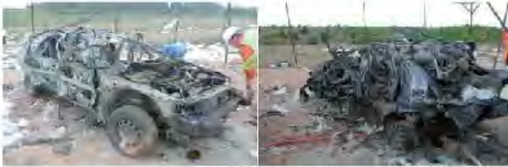
Figure 4.1 Damage to cars placed inside a detonating propane-air cloud [32]
