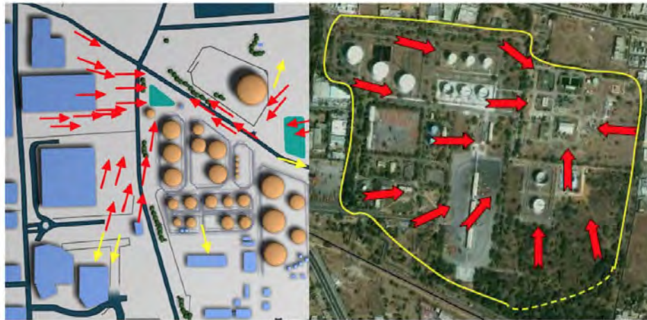
Figure 4.10 Examples of directional indicators found in the detonation incidents at Buncefield (left) [1] and at Jaipur (right) [4]. The yellow boundary on Jaipur marks the edge of the vapor cloud.
