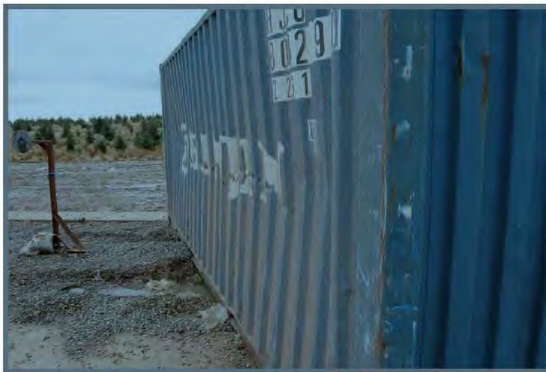
Figure 4.6 Damage to an iso-container when the incident overpressure was 2 atm (photograph reproduced from [32]).
