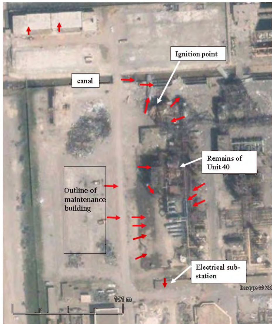
Figure 5.3 Directional indicators derived from photographic evidence of the Skikda explosion (Google Earth image with overlays).
