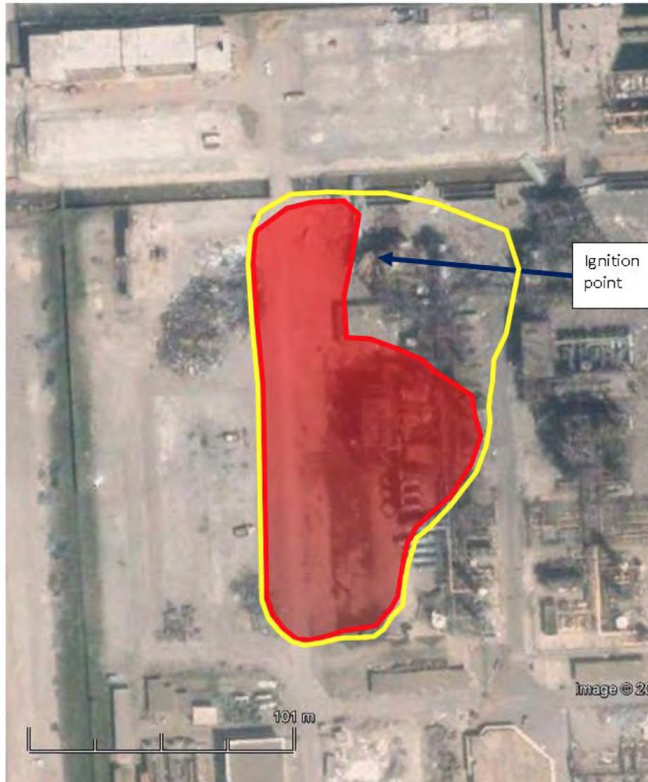
Figure 5.4 Proposed area of detonation (red) and cloud size (yellow boundary) (Google Earth map with overlays).
