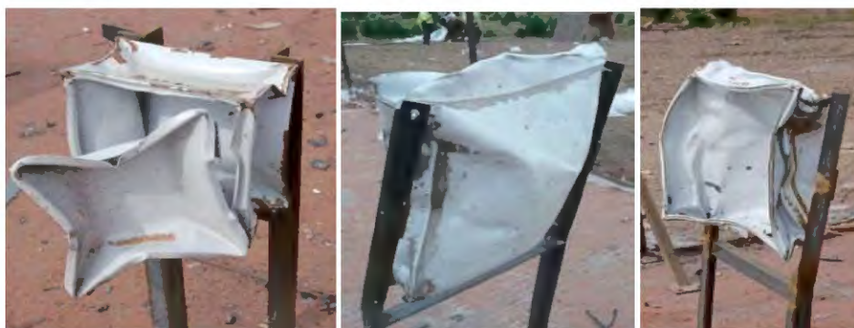
Figure 4.4 Damage to small and large instrument boxes placed inside the detonation, (photographs reproduced from [32]). Left figure: A small box, 30 cm \times 30 cm. Middle figure and right figures: Two views of a larger 60 cm \times 60 cm box.
