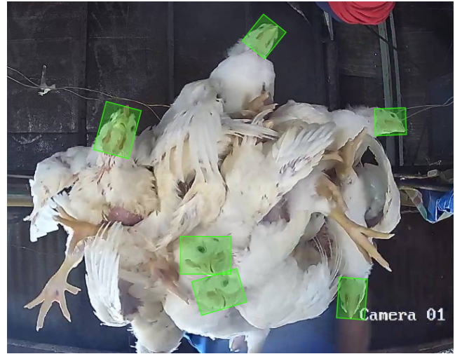
Fig. 3. Example annotated harvest-stage frame illustrating the broiler-head target under overlapping birds, partial occlusion, and irregular head orientations.
