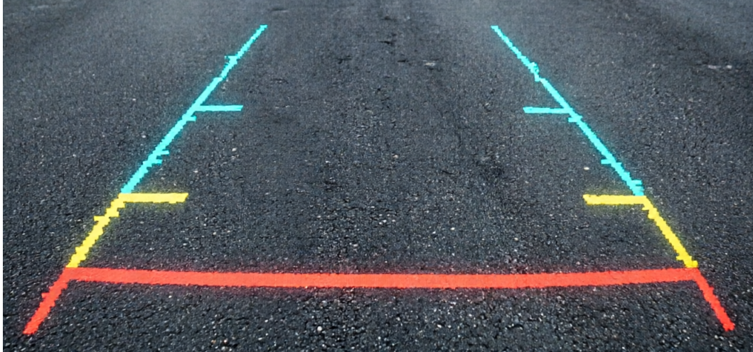
Figure 1: Parking guidelines without MSAA. Diagonal segments show visible staircase aliasing (rated 1.4/5 by observers), especially on the converging lines. The camera feed (wet pavement background) does not exhibit aliasing because it is a video texture, not rendered geometry.
