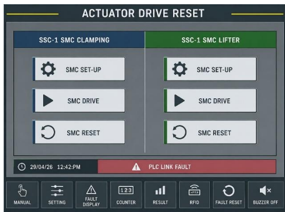
Figure 4 HMI fault recovery screen
