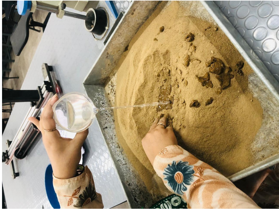
Figure 16 : ADDING WATER INTO SOIL
