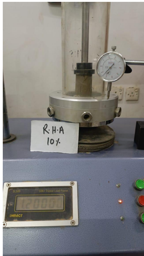
Figure 49: APPLYING LOADING ON SAMPLE WITH 10% RHA
