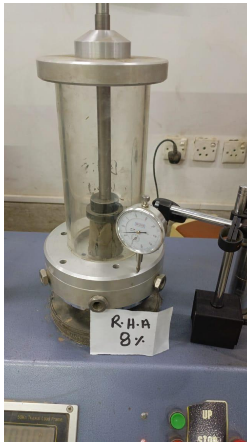
Figure 47: APPLYING LOADING ON SAMPLE WITH 8% RHA
