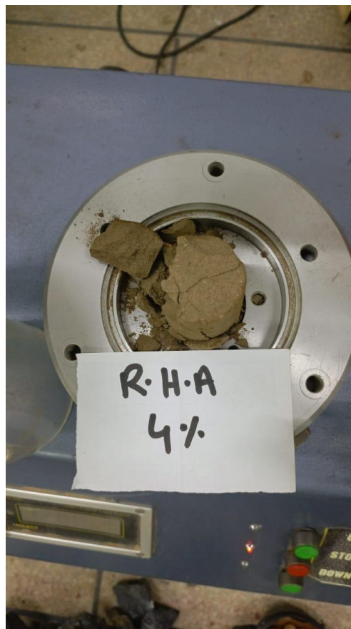
Figure 45: AFTER LOADING ON SAMPLE WITH 4% RHA
