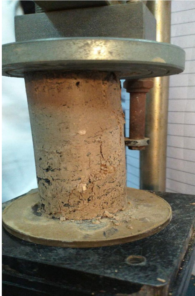
Figure 27: APPLYING LOADING ON BITUMEN SAMPLES
