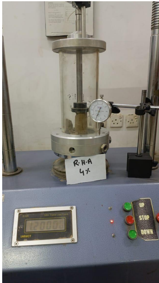
Figure 43: APPLYING LOADING ON SAMPLE WITH 4% RHA
