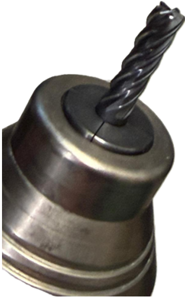
Figure 5. Tool-failure event (Topcut, 6-flute, S688, 1 mm, F296): (left) fractured end-mill tip; (right) the corresponding force record.
