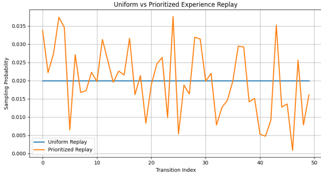
(a) Comparison between uniform replay and prioritized replay sampling distributions. Under prioritized replay, transitions with larger temporal-difference errors receive higher sampling probability: P(i) = \frac{p_i^\alpha}{\sum_{j=1}^N p_j^\alpha} , p_i = |\delta_i| + \varepsilon . The figure illustrates how prioritization allocates more computational effort to informative transitions.
