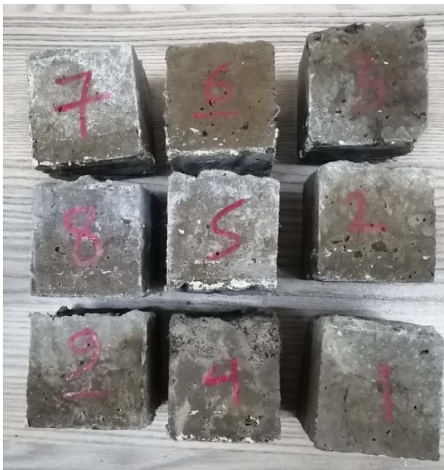
Figure 13. Visual appearance of the magnesium sulfate-cured geopolymer composite samples
