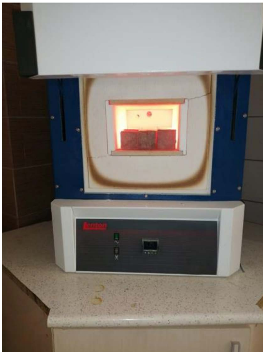
Figure 3. Furnace with 1200°C temperature
