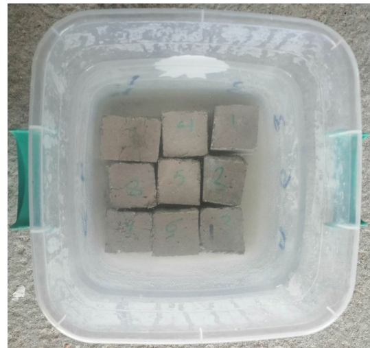
Fig. 9 Specimens exposed to magnesium sulphate solution
