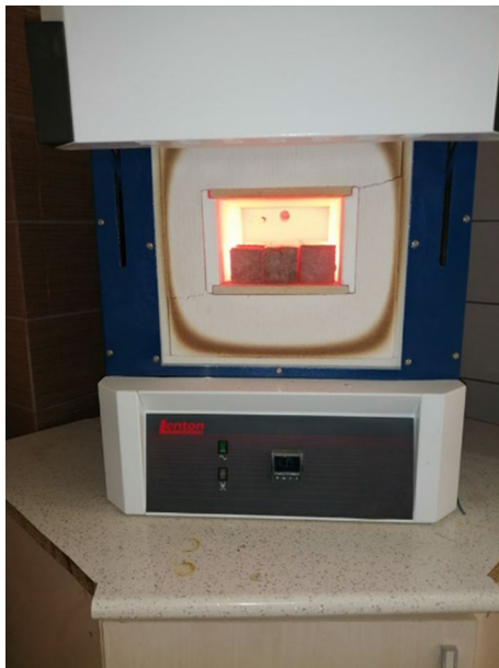
Fig. 7 Furnace with 1200 °C capacity to evaluate the fire resistance of AAM
