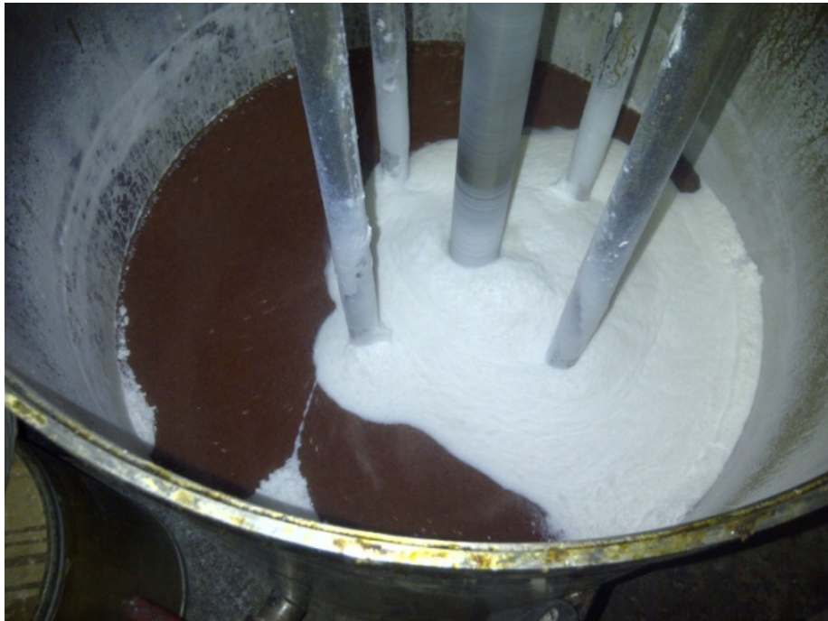
Figure 1: Cowell's Disperser for mixing.
