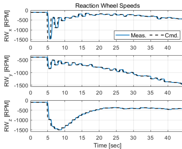
Figure 19. Reaction wheel speed commands and measured wheel speeds during the three-axis diagonal maneuver.
