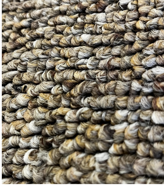
Figure 11: Close-up of the loop-pile apartment carpet surface showing directional fiber grain texture. The anisotropic fiber orientation creates direction-dependent friction on the 45° angled mecanum rollers, producing the CW/CCW rotation asymmetry observed in Figures 12 and 13.
