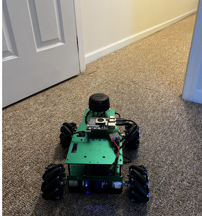
Figure 9: Test environment showing the robot at the bedroom-to-hallway doorway (0.76 m width) on loop-pile apartment carpet. The carpet fiber texture and doorway clearance relative to the robot chassis are visible.
