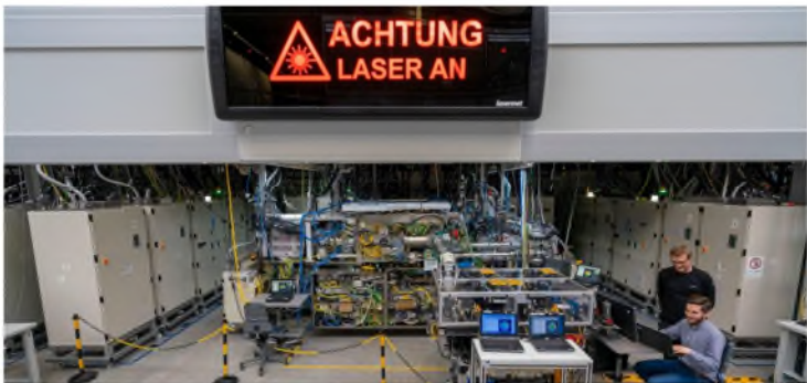
Plate III: Sub-Fab Infrastructure: High-Power Laser Source and Beam Delivery Unit (BDU). Description: The massive underground support level situated directly beneath the cleanroom floor. This area contains the multi-stage TRUMPF pulsed CO 2 laser seed oscillators, industrial optical power amplifiers, and the rigid BDU pipeline that routes the infrared "photonic pump" toward the tin droplet generator core.
