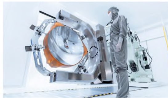
Plate IV: The Zeiss SMT high-NA EUV mirror, featured as Plate IV, utilizes specialized atomic layering for high-reflectivity molybdenum-silicon coatings within a cleanroom environment. Technical specifications include a 6-ton illuminator optics box with 25,000 components and a 12-ton projection optics box (POB) containing 40,000 components, totaling 18 tons of optical assembly. Learn more about Zeiss SMT's manufacturing technology at ZEISS SMT .
