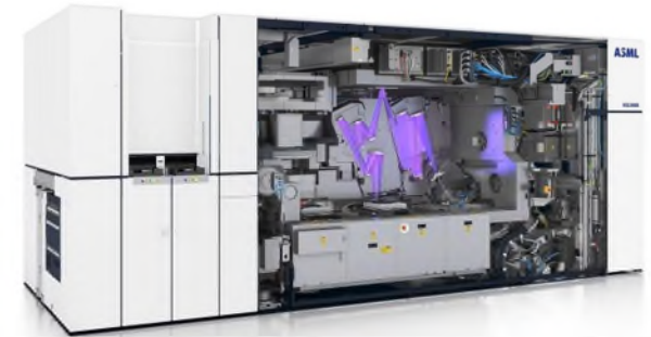
Plate V: Optical Path of the Illumination System and the Projection Optics Box (POB) Description: Internal three-dimensional schematic of the central scanner core, mapping the complete reflection sequence across the Carl Zeiss SMT mirror assembly. Note: The colored rays tracing the path from the illuminator system through the reflective reticle and into the anamorphic POB are digitally rendered for illustrative clarity; the actual extreme ultraviolet (EUV) radiation operates at a nanometric wavelength 13.5 nm propagating entirely within an ultra-high vacuum (UHV) environment and remaining physically invisible to the human eye.
