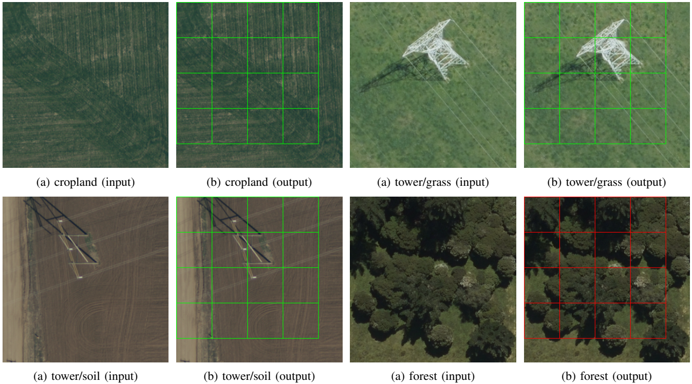
Fig. 10. Example inputs and predicted outputs. For each scene, (a) is the raw RGB input patch and (b) is the classifier output, where the patch grid is coloured by predicted class ( green = low-density, red = high-density vegetation flagged as potential encroachment). The three low-density scenes—cropland, a transmission tower over grass, and a transmission structure over bare soil—are correctly passed (green), with towers and conductors causing no false alarms, while the dense forest scene is correctly flagged (red).
