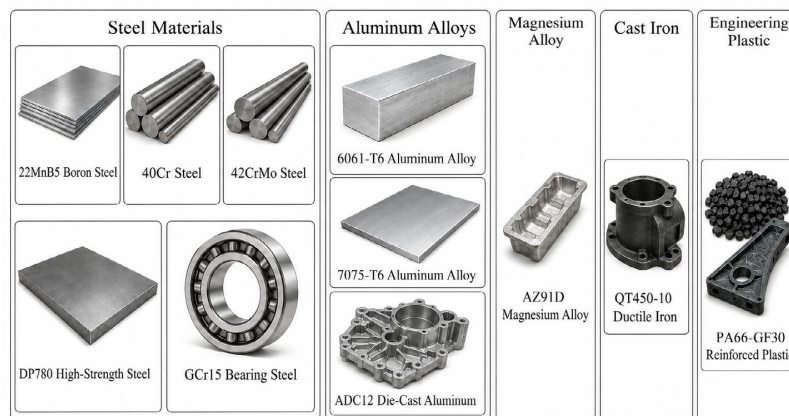
Figure 1: Material type grouping diagram for automotive component forming quality prediction
