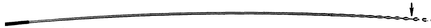
FIG. 9: Photograph of a water jet in the laminar Rayleigh regime from Grant (1965, fig. 5-3a). Note the breakup is caused by disturbances symmetric to the jet axis. The arrow indicates the location of breakup. Flow is from left to right.
